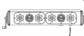
Use the 8mm X 12mm bolts (5) to attach the mounting legs. Mounting legs (3) can be installed in ether direction depending on space constraints. When mounting with opional clamps (PR-URM, PR-FRC200, and PR-FRC175) use the hex bolts provided with the clamps to mount the bottom half of the clamps to the mounting legs.
