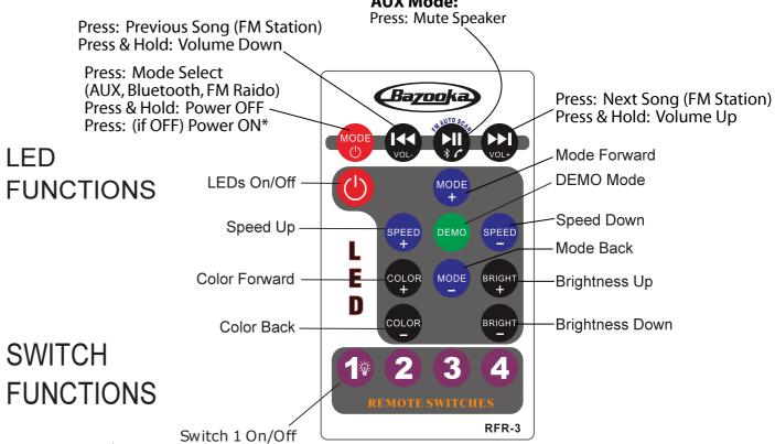
Remote switch buttons 2-4 are not used with this model
